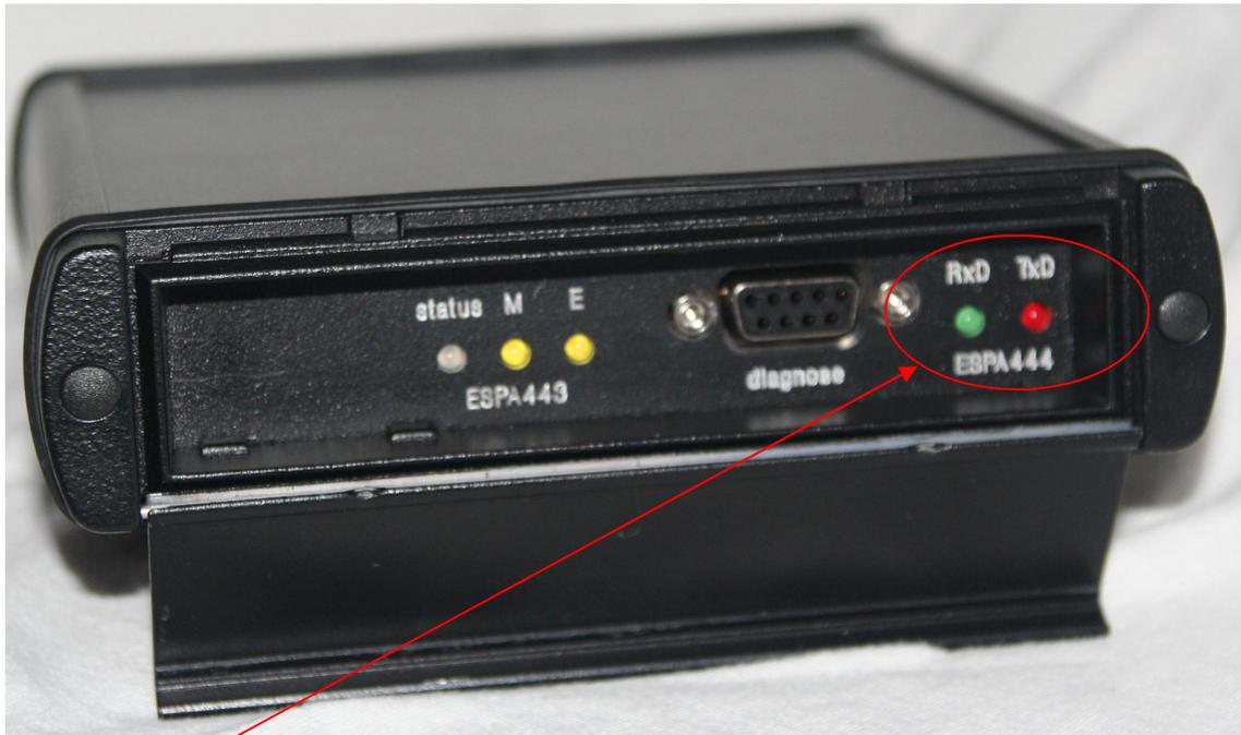
The TxD and RxD leds indicate the communication on the RS232 serial lines to the ESPA 4.4.4. device. If data is sent, the red led lights up shortly, if data is received the green led lights up shortly.
