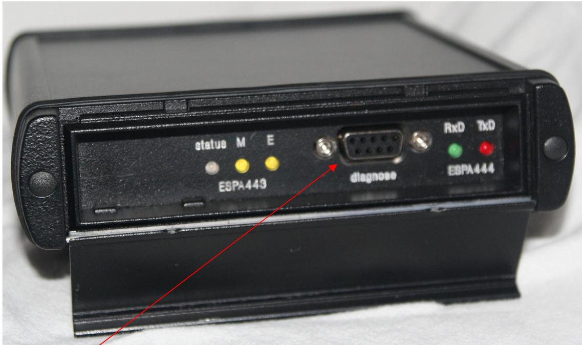
If needed, the converter can be setup with a 'ConfigTool'. This is a program running under Windows XP, Vista, 7 and 8 using the serial port of a computer or a laptop. It can be used to program settings into the converter, reading current settings out of the converter and to read serial diagnose information
