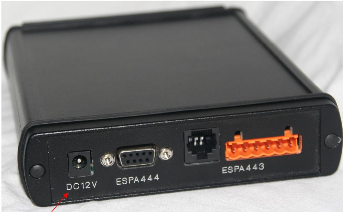
The power supply of the converter is 12V DC.
