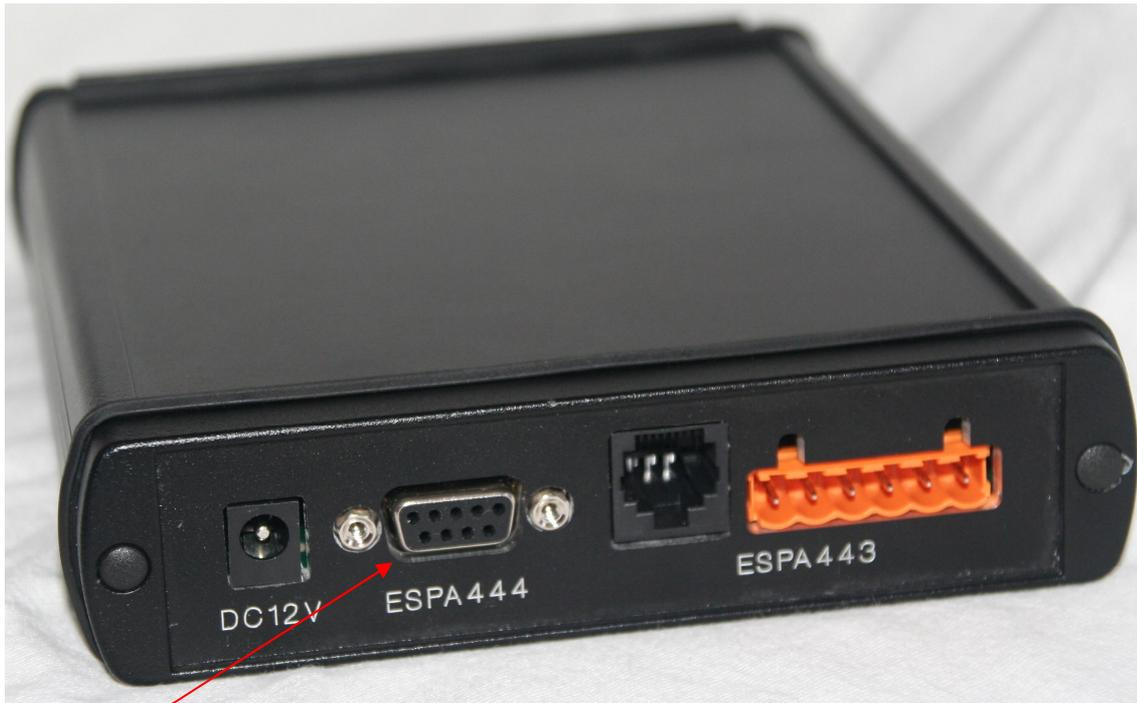
The converter uses a standard 9 pole SUBD connector with RS232 to communicate with its peripheral (PC or other system).
