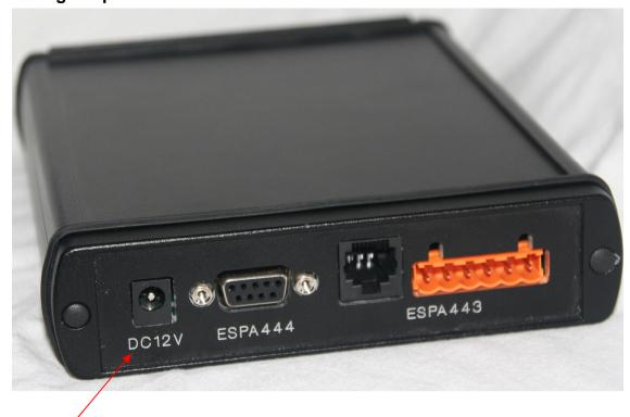
The power supply of the converter is 12V DC. Please us the supplied power supply.
