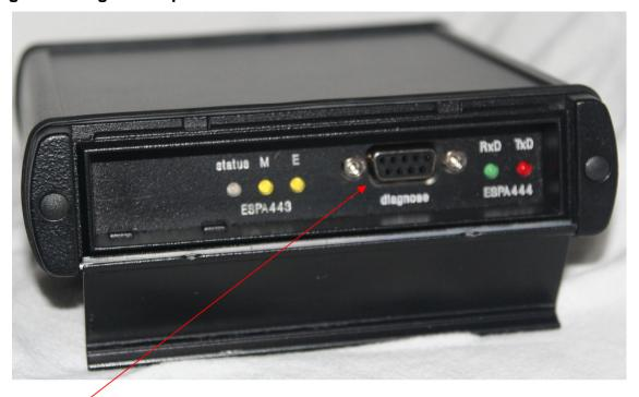
If needed, the converter can be setup with a 'ConfigTool'.
