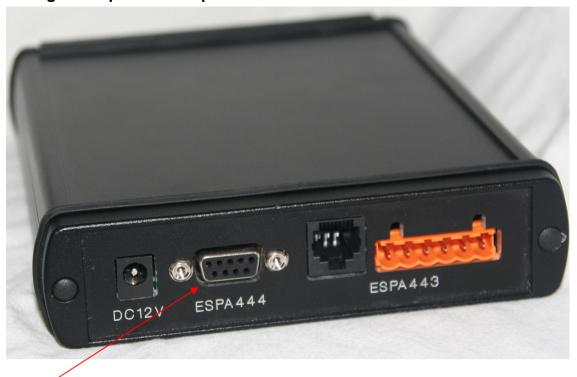
The converter uses a standard 9 pole SUBD connector with RS232 to communicate with its peripheral (PC or other system).
