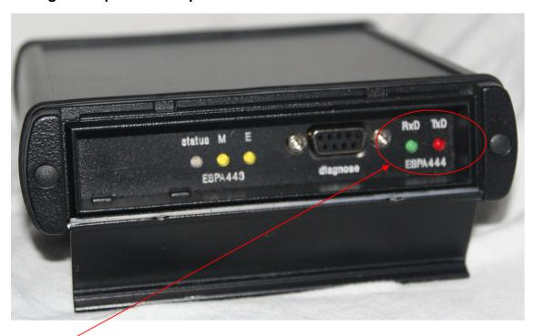
The TxD and RxD leds indicate the communication on the RS232 serial lines to the ESPA 4.4.4. device. If data is sent, the red led lights up shortly, if data is received the green led lights up shortly.
