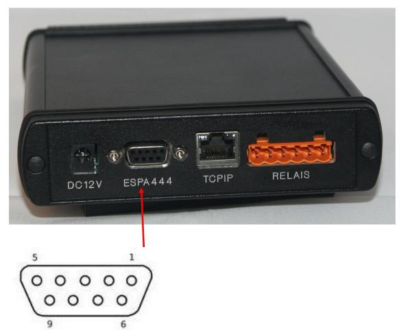
The convertor uses a standard 9p SUBD connector to connect to the ES-PA444 equipment.
